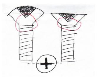
I believe the 'domed' type screw is far superior to the 'flat' type. Originally I thought the previous owner changed the screws for whatever reason. However I recently found the same screws fitted to another P76 a mid 74 Executive. So it would seem there were at least two different types used during manufacture.
